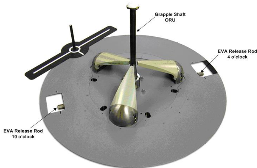
FIGURE E.1.2-1 FLIGHT RELEASABLE GRAPPLE FIXTURE
